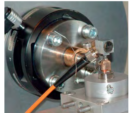
Load testing of a double crown.
