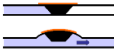
Working principle of a diaphragm valve. Usually, valve applications require higher forces than pumps.
