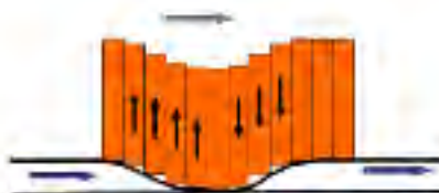
The principle of peristaltic pumping makes directional valves obsolete; the pumping direction in this case is specified by the order in which the individual actuator elements are driven.
