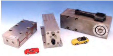
Several PZT driven tool servos (match box cars and connecting rod for size comparison)
