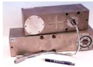
Fast Tool-Servos with Solid State Piezo Drives (excentric machining of pistons)
