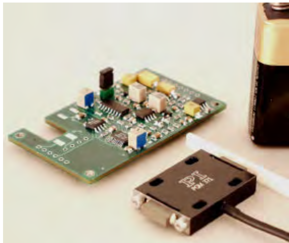
Fig. 5: Drive module, friction bar and drive electronics (9-V battery for size comparison)
