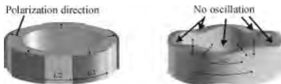
Fig. 5: Piezo cylinder deformation, electrode arrangement, polarization and end-point motion for the 5th degenerate coupled axial-tangential mode
