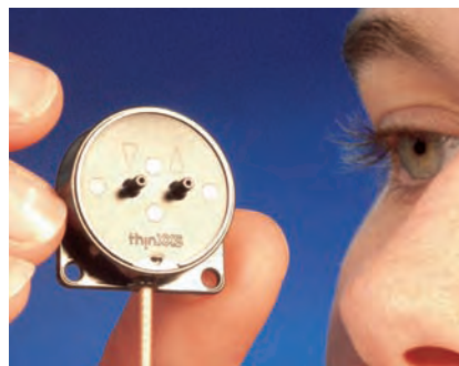
Custom piezo disks precisely dose liquids and gases in the ThinXXS micropump. (source: thinXXS Microtechnology AG)
