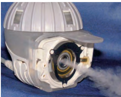
An annular piezo disk serves as an ultrasonic transducer to produce the aerosol in the atomizer head of the eFlow® rapid Electronic Nebulizer series. (source: Pari Pharma GmbH)
