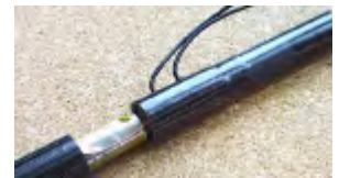
Actuator embedded in carbon fiber rod (smart structure, active vibration cancellation)
